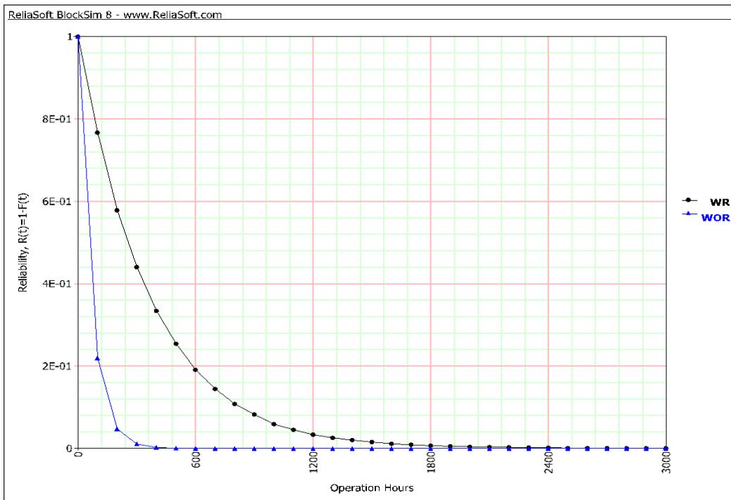
Figure 5. Binary system reliability of power generation system with redundancy (WR) and without redundancy (WRO)
