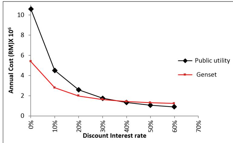
Figure 15. Effect of interest rate on redundancy evaluation
